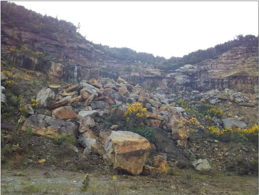
Figure 3 Active face with material available for removal
